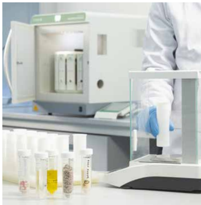
1 - Weighing step on the hydrolysis/ extraction vessel
